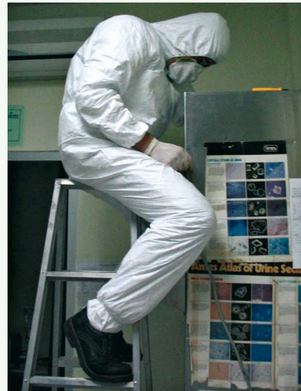
Jan Jacobs providing technical assistance to the laboratory of the Sihanouk Hospital Centre of Hope (Phnom Penh, Cambodia): replacing the HEPA filter of a biosafety cabinet.
