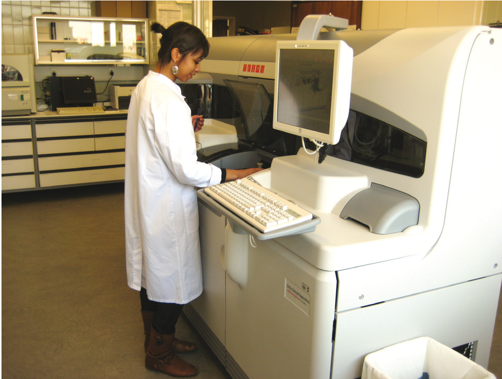
The integrated analyzer replaces four different machines.
